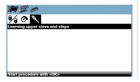
Learning zero returns volume and setting the returns volume limit calibrate the return elevator
