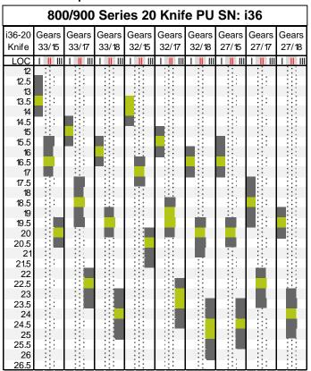
The CLAAS Green box is for best sprocket ratio for a LOC. The CLAAS Dark Grey is for acceptable sprocket ratio for a LOC. Note: half link is required for some sprocket combinations not provided with head.
