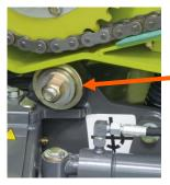
The auger down stop rollers have 2 positions for adjusting auger height.
