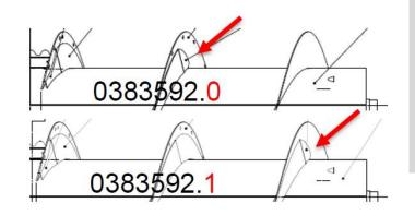
The auger flights are now reinforced up to the end of the auger
