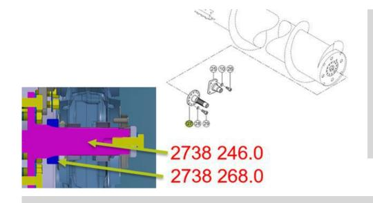
From BY 2020 all machines are equipped with a reinforced drive flange
